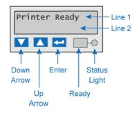
3 Press the Up or Down Arrow key to scroll to "Data Format" and press the Enter key.
