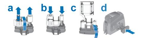
6 Load cards in the input hopper (if the printer has a hopper).
